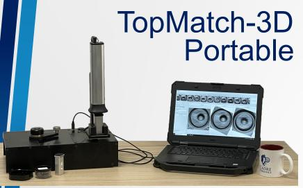
Introducing the latest addition to Cadre's courtroom-proven VCM platform - the newly redesigned Portable Scanner. The Cadre TopMatch-Portable system uses the same gel technology as our validated desktop system to capture high-resolution, traceable 3D surface topographies. With a lateral spacing interval of approximately 2.75 microns per pixel, the portable unit provides accurate scans that can be analyzed with the same TopMatch software as the desktop system
